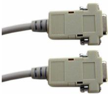
**Interface cable, RS232, crossed wired (null modem cable)**
